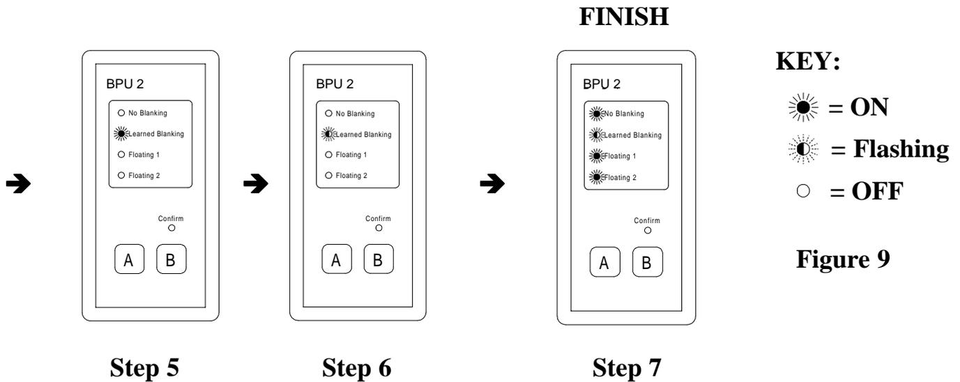
5. To program a particular mode, press buttons A and B together for 3 seconds when the desired mode indicators are ON.
