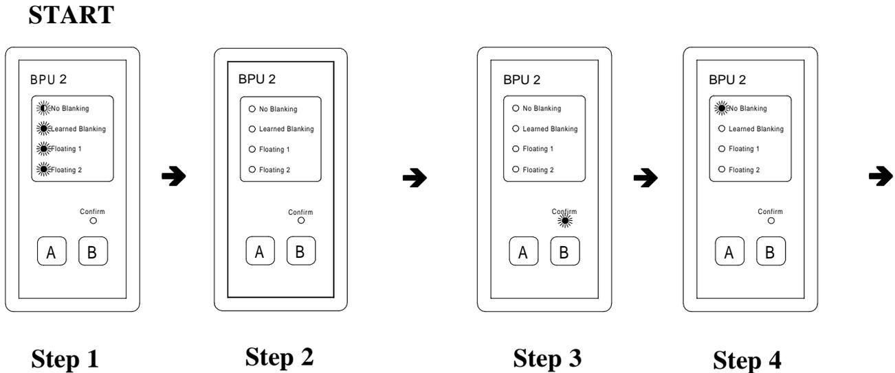
1. Connect the programming unit in-line with the receiver unit. All the mode indicators will come ON with the current mode indicator(s) flashing.
