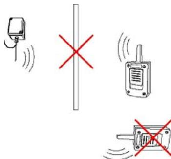
The transmitter and receiver antennae must be parallel to each other for optimum signal reception
