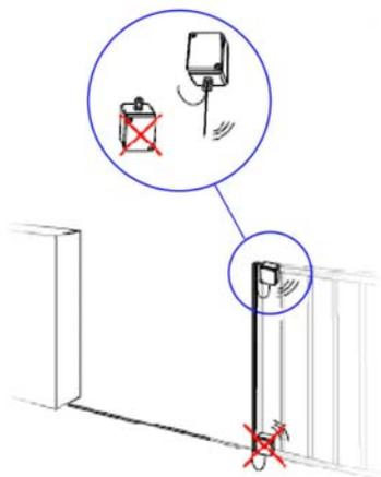
Install the equipment so that the cable gland is at the bottom. In installations that could possibly have range problems between the transmitter and receiver, ensure that the antenna hangs vertically from the hole in the cable gland.
