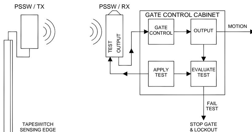
and checked by the gate/door control unit before every operation. If the outputs fail to respond, the operation of the gate/door should be prevented until the situation is corrected. The auto-test can be applied by a signal connected to ATEST1 (for output R1) and/or ATEST2 for (output R2). Only apply the auto-test for outputs that are being used. . The PSSW/RX can deal with positive- or negative-polarity auto-test signals applied by the gate control cabinet.
