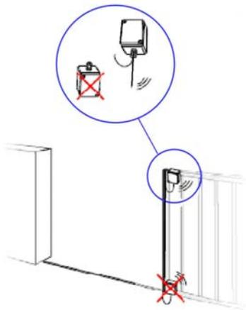
Install the equipment so that the cable gland is at the bottom. In installations that could possibly have range problems between the transmitter and receiver, ensure that the antenna hangs vertically from the hole in the cable gland.
