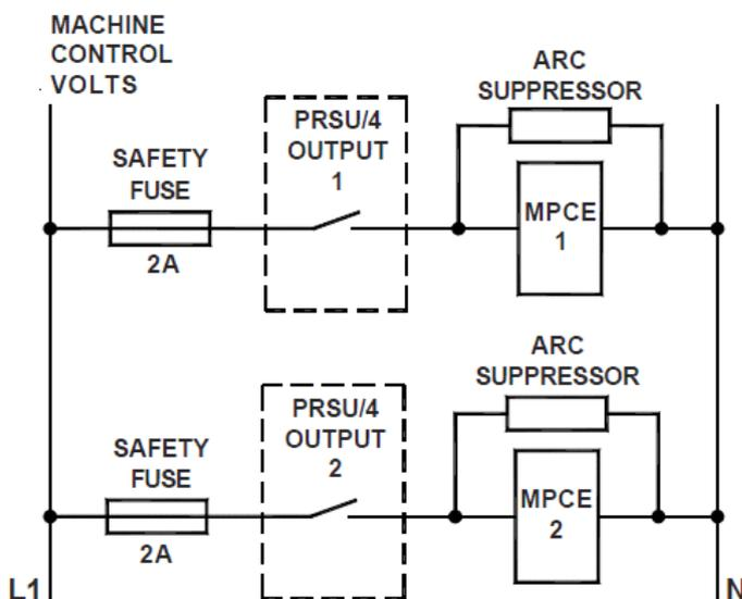
**Figure 22– Safety Output Connection (Two MPCEs)**
