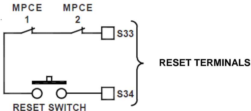
Figure 20– Cross Monitoring of MPCEs
