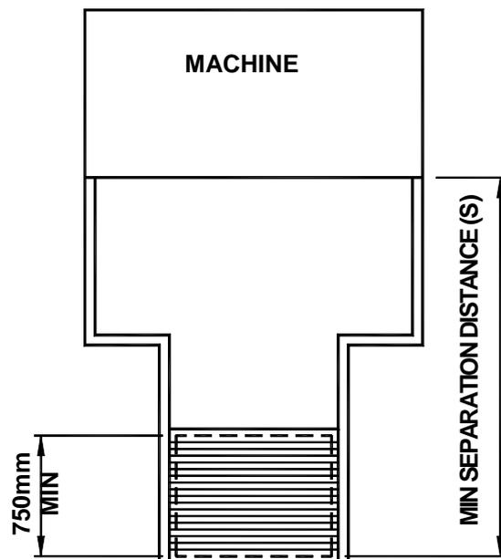
Figure 6—Mat solely used as a trip device
