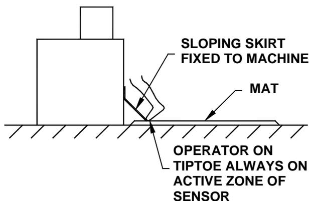
**Figure 11 - Ensure operator is always standing on active area of sensor**
