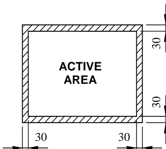
**Figure 1 - Dimensions of the inactive area around outer edge of sensor**
