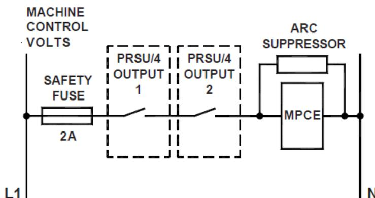
**Figure 21– Safety Output Connection (single MPCE)**
