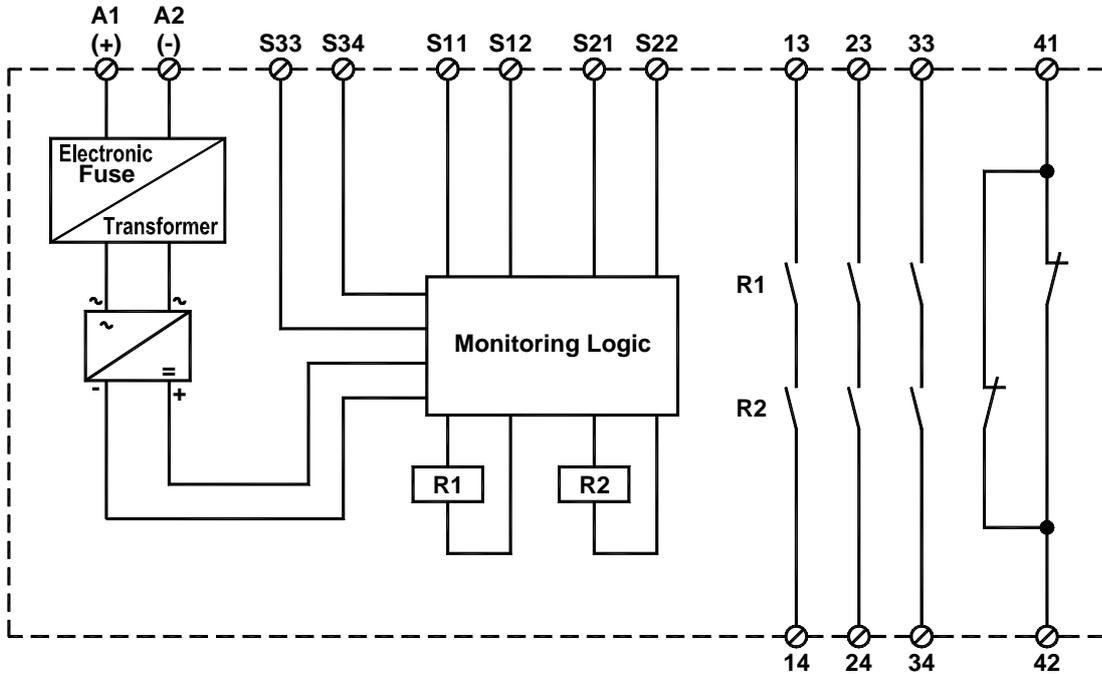
Figure 17 - Control unit connection
