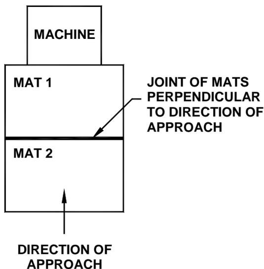
**Figure 3 - Arrangement of mat joints**
