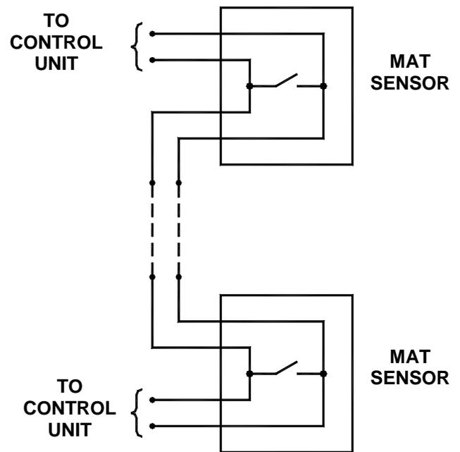
**Figure 10-Construction of sensors in series**
