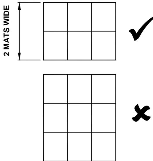
**Figure 4 - Mat array requirements**
