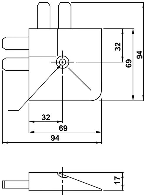
**Figure 13 - AE-C Corner piece**
