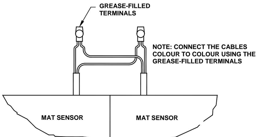
**Figure 16 - Wiring of two mat sensors each with 2 x 2 core cables**
