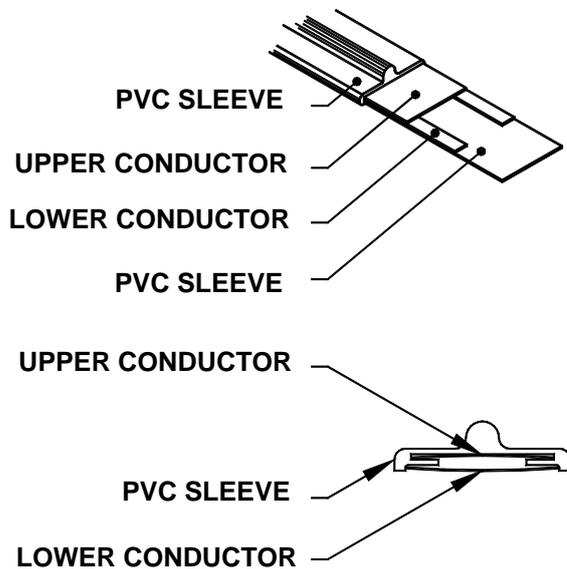
**Figure 9 - Construction of Tapeswitch elements**
