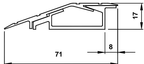
**Figure 12 - AE-13 Sensor Edging**
