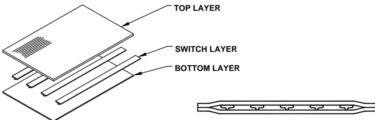
Figure 8 - Construction of CKP/S1 sensor
