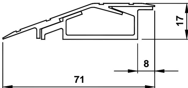
**Figure 6 - AE-13 Sensor Edging**
