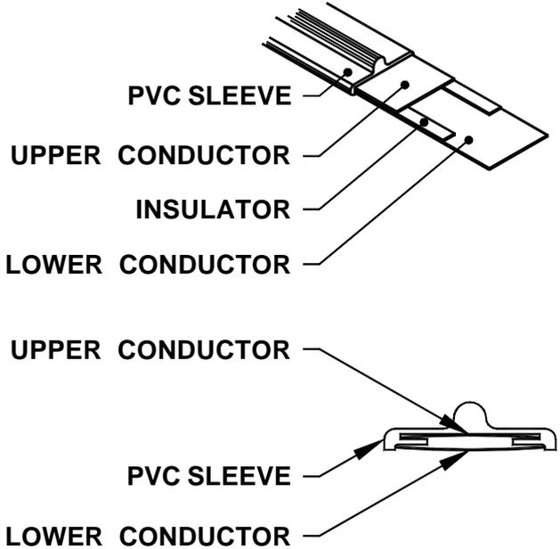
**Figure 3 - Construction of Tapeswitch Switch Elements**
