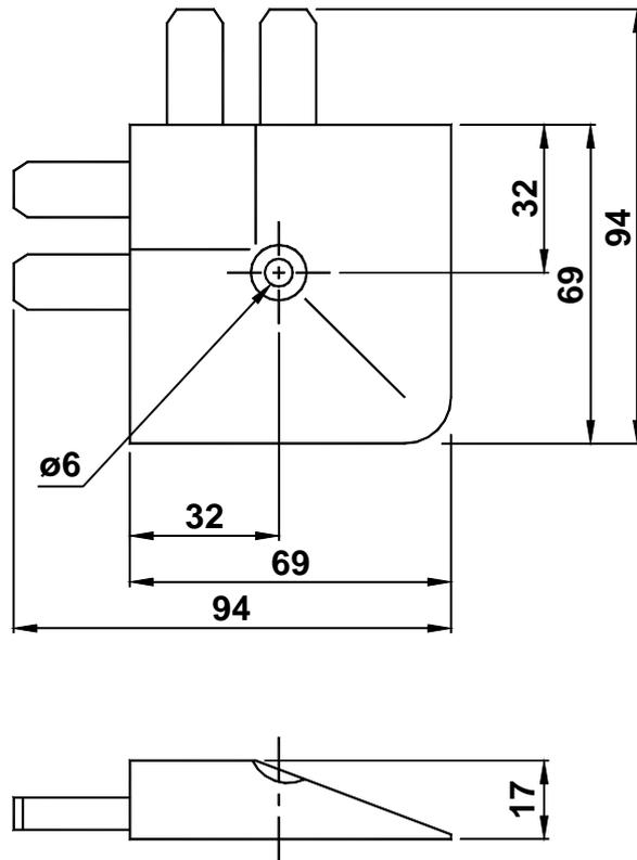
**Figure 7 - AE-13 Sensor Edging**
