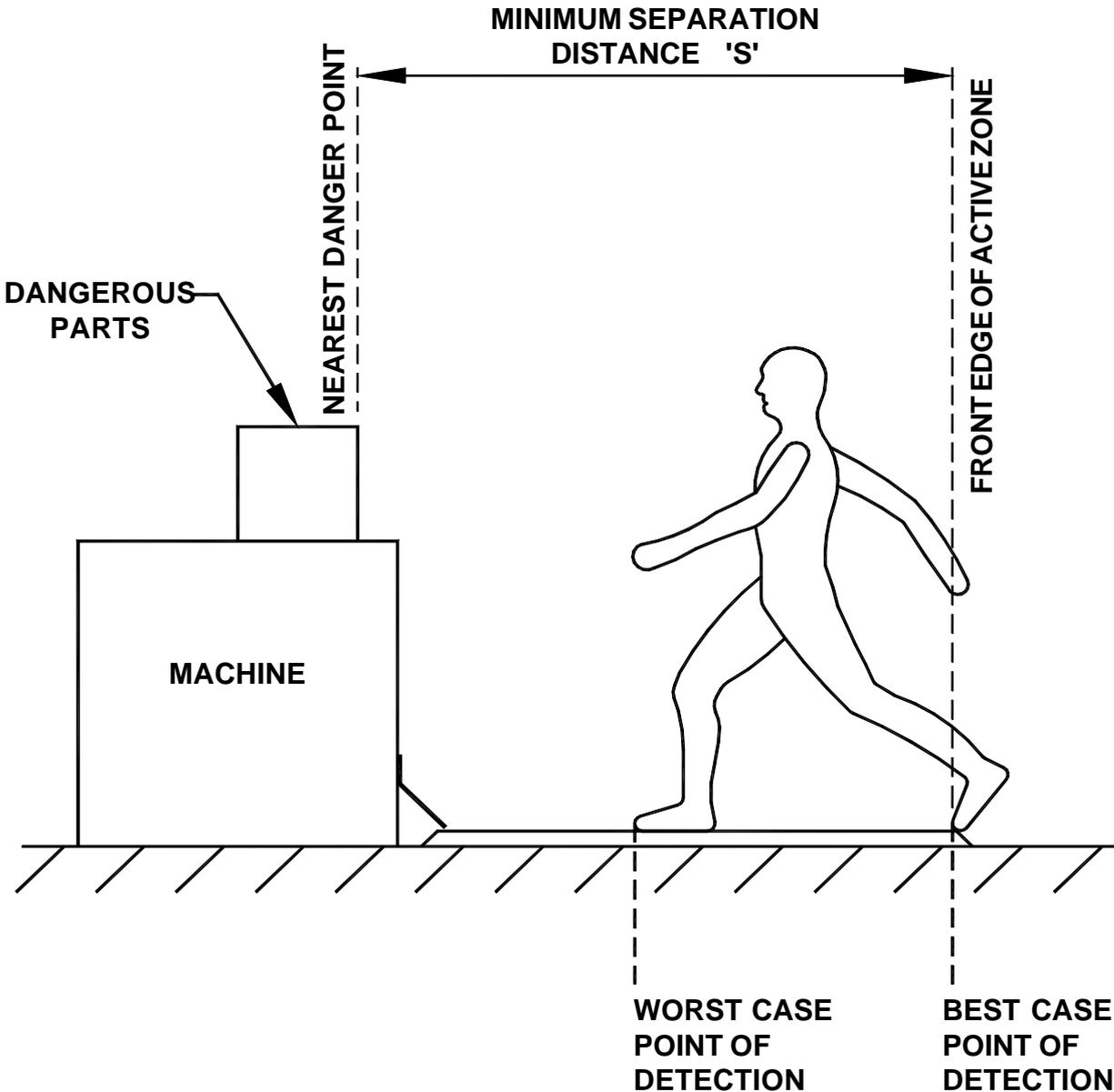
Figure 4 - Minimum Separation Distance
